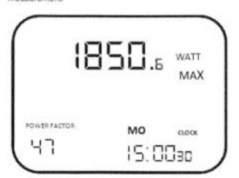
Press the MODE key to switch to the kWh (kilowatt hours) range. Here you can check the previously measured power of the consumer in kWh, power factor, weekday and the current time.
