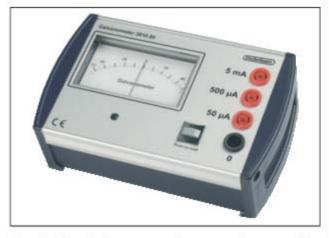
The Student Galvanometer is a rugged yet sensitive instrument, designed specifically for student experiments. It has a center-zero meter and three current ranges. When performing a null-current experiment, such as measuring resistance using a Wheatstone bridge, it is easy to balance the current using the 5 mA range, then step down through the lower current ranges to very accurately determine the point of zero current.
